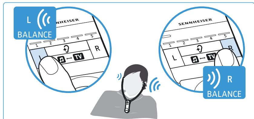
To reset the balance setting to the middle setting:
