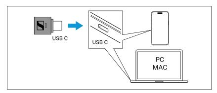
▷ Connect the dongle to a USB C socket of your mobile device or PC/Mac.
