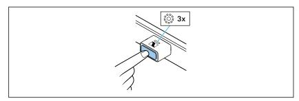
During the connection attempt, the status LED of the dongle flashes white 3x repeatedly. The connection process can take up to 20 seconds.
